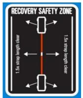
zone of both helpers & watchers before the actual pull begins. If you are operating a winch, position yourself in a safe position such as inside the cab or behind the door. If repositioning is needed, in the middle of a recovery, always loosed tension on the pull line before entering the danger zone.
