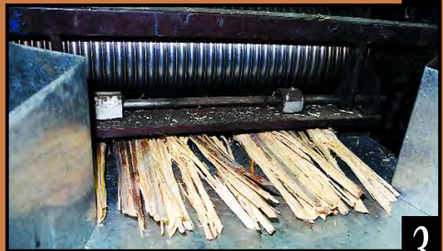
The crushed logs are processed into scrim—long, thin lengths of wood.
