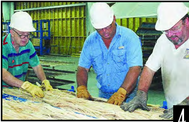
The scrim is placed on trays for drying
