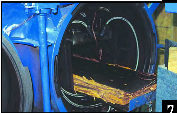
Scrim is then placed in the patented steam injection press.
