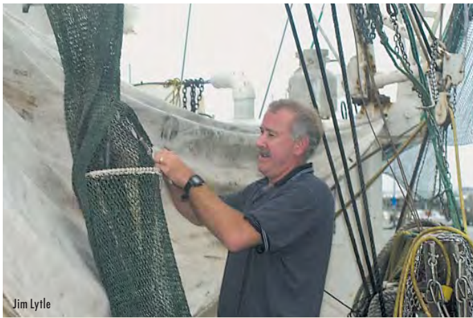
Marine resources specialist Dave Burrage installs a bycatch reduction device into a shrimp net.
