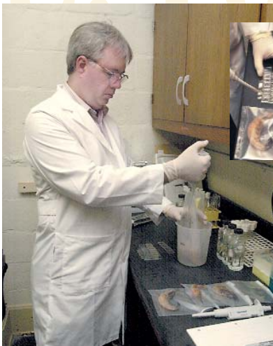
MAFES food scientist Douglas Marshall prepares a sample of shrimp for bacterial analysis using impedance technology.
