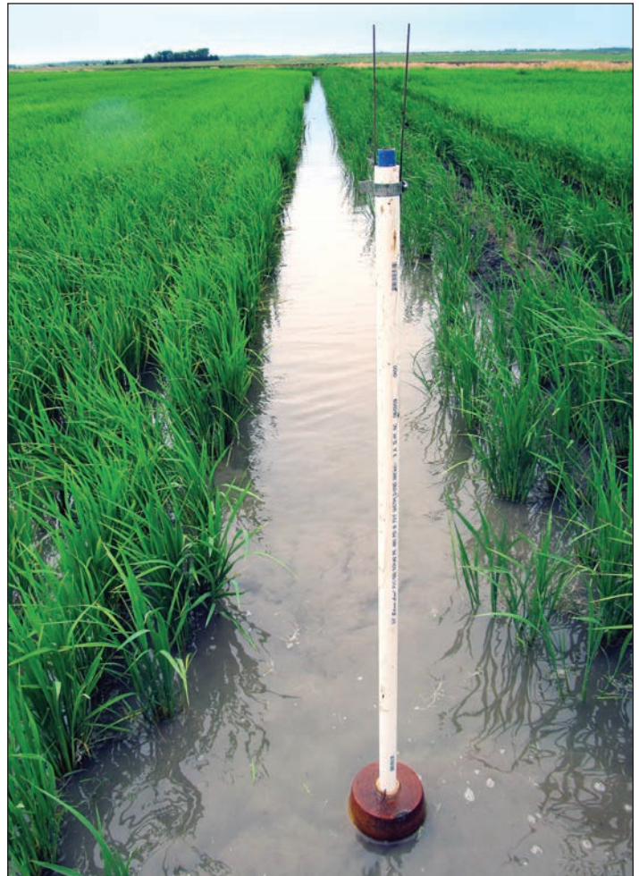
Figure 1. A simple rice flood depth gauge can help to save water, time, and money.
