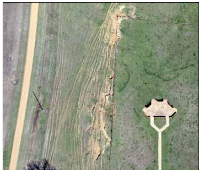
Figure 11. Image of erosion within the Catalpa Creek watershed taken from an unmanned aerial vehicle.
