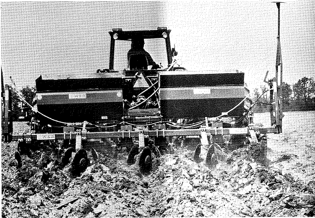
Figure 4. Applying dry lime in acid subsoil.
