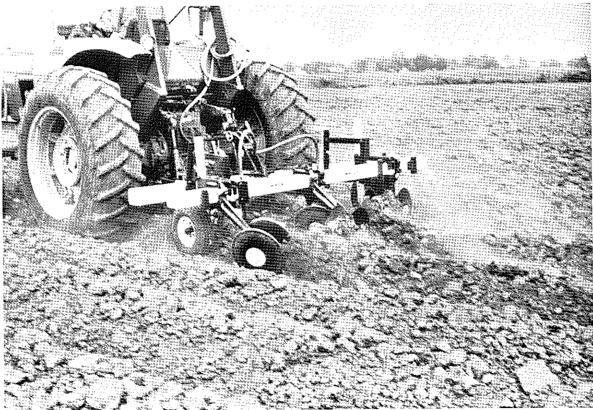
Figure 2. Applying suspension lime in acid subsoil.
